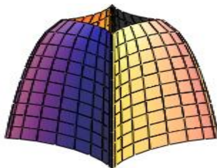
Fig. 8. An umbrella-type service with astroidal lines of level formed by biquadratic parabolas
