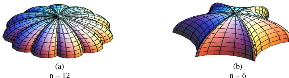
Fig. 6. Umbrella-form surfaces with a contoured spherical surface: (a) a sphere with external cycloid crimps; (b) a sphere with inner cycloid crimps
